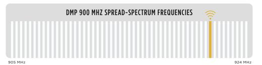
DMP Two-Way Wireless alarm systems operating in the 905-924 MHz spectrum band offer numerous advantages over other products. These include:
